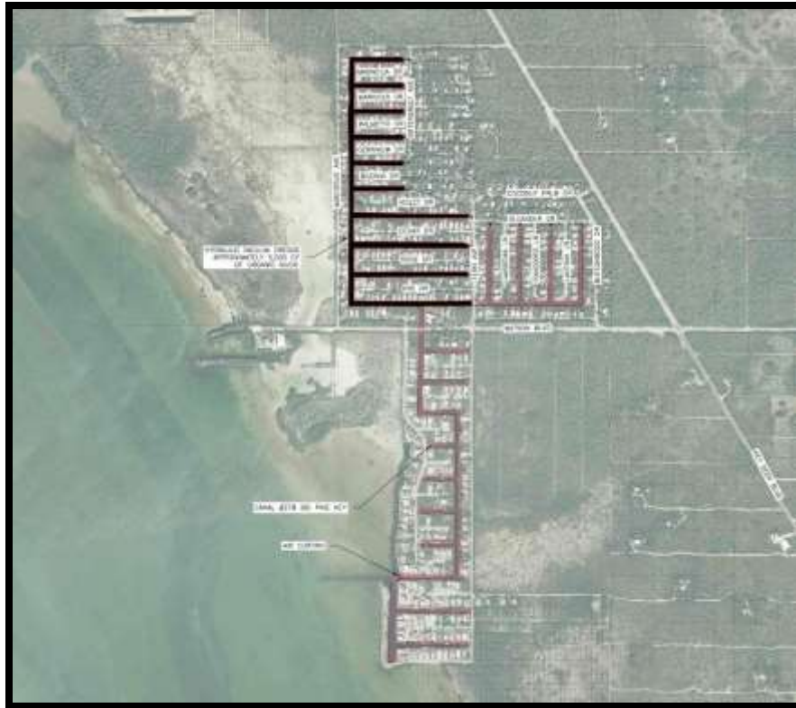
Figure 11 – Conceptual Layout for Organic Sediment Removal
