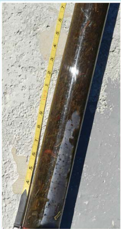
Due to persistent currents and wind direction, a thick weed wrack becomes entrapped in the canal and sinks to the canal bottom where it decays.
