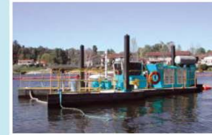
The utilization of a hydraulic vacuum dredge will result in the collection of a wet slurry from the canal bottom comprised of decaying organic matter and saltwater.
