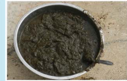
The utilization of a hydraulic vacuum dredge will result in the collection of a wet slurry from the canal bottom comprised of decaying organic matter and saltwater.
