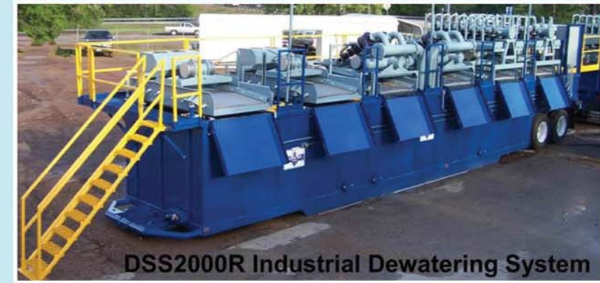
In order to expedite the dewatering of the dredged slurry, polymers will be added to the slurry prior to its temporary storage in a mechanical dewatering press.
