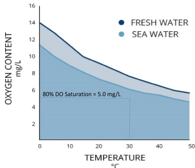
Figure 2. Dissolved oxygen concentrations as temperature increases for freshwater (top line) and saltwater (bottom line). Credit Fondriest
