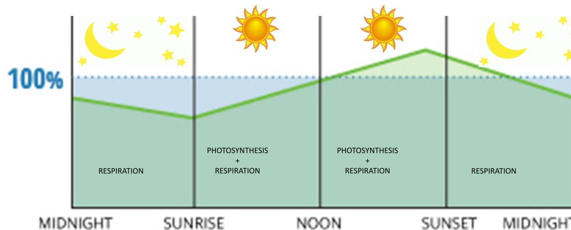
Figure 4. 24 hour (diel) variations in dissolved oxygen levels due to photosynthesis and respiration. Credit Fondriest
